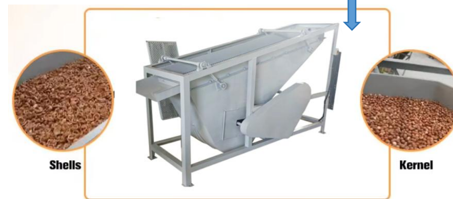
Sieve shells and kernel Separator separates shell and kernel
