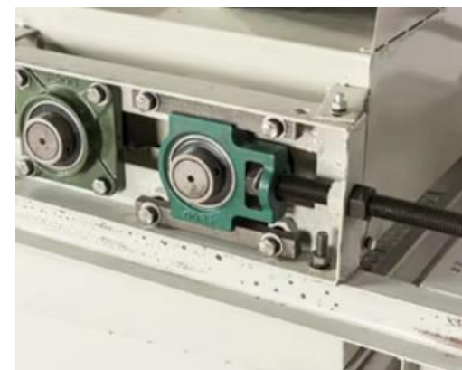
Observe the changes in the rollers and the size of the gap
